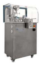
Lab scale automated capsule liquid filling and sealing machine, combined in one piece of equipment with a nominal throughput of 1,500 filled and sealed capsules per hour.
