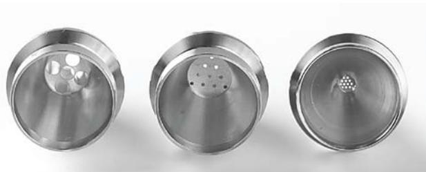
Even with a sufficiently finely divided powder, a dispense head (image of 3 dispense heads above) must be selected so that the amount released per tap is small compared to the target dose amount. In principle this is achieved by a suitably fine mesh, and so we constructed special dispense heads to test if this was a limiting factor in practice for dispenses down to 10µg.
