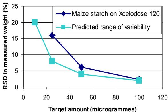
The graph above shows the predicted range of variation for an Xcelodose system set up with a 1 $\mu$ g stability range. The experimental data is from runs using the same parameters with 100% pass band.
