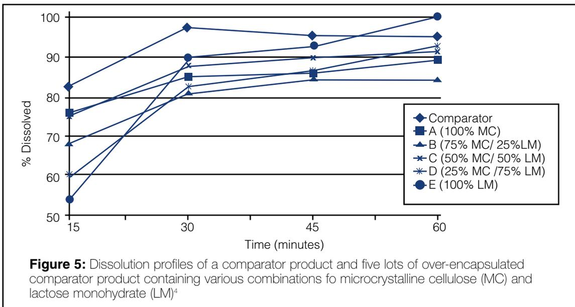
**Figure 5:** Dissolution profiles of a comparator product and five lots of over-encapsulated comparator product containing various combinations fo microcrystalline cellulose (MC) and lactose monohydrate (LM)<sup>4</sup>
