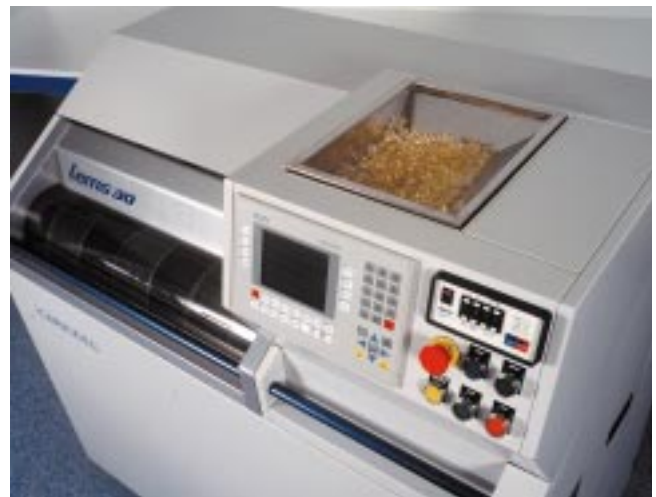
Figure 4: LEMS™ 30 machine for sealing hard gelatin capsules.
