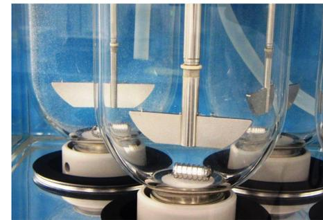
To evaluate the behavior in the presence of 40% ethanol in the dissolution test the double capsule options were tested at pH 1.2 USP with 40% ethanol using dissolution test equipment Sotax AT70 USP apparatus 2, caffeine 100mg formulation and dissolution sinker.
